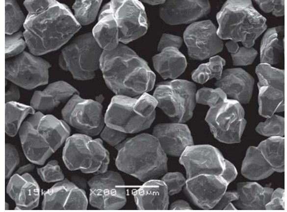
Fig. 3. Tungsten powder was imaged using a JEOL 6060LV general purpose scanning electron microscope. The powder is sold as Technon Tungsten Powder 100 mesh, with 90% of the particles ranging in size between 25 and 150 \mu\text{m} . This wide distribution allows for higher packing density within each block.
