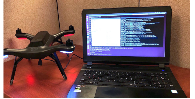
Figure 13: Emulation mode where FlyNetSim is run on-board a 3DR Solo UAV.
