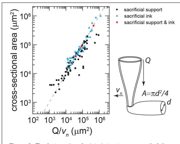
**Figure 2.** The feature size of printed structures generally follows the scaling predicted from the material deposition rate ( $Q$ ) and printing nozzle translation speed ( $v_n$ ) using volume conservation. Dashed line:  $A = Q/v_n$  with no adjustable parameters. Data were collected from a survey of literature reporting on soft matter 3D printing methods and materials.<sup>1,3,4,12,22,27,29–32</sup>
