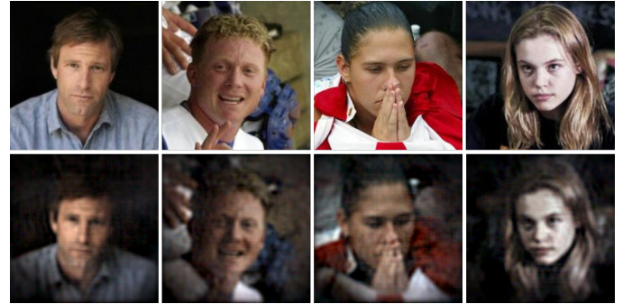
Fig. 3: Images from the LFW dataset (top) were displayed on a screen and then captured and reconstructed (bottom) by FlatCam. The lensless reconstructions feature artifacts and non-idealities that are not present in standard camera images.
