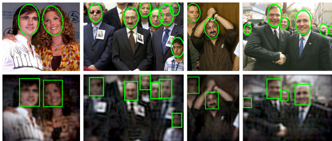
Fig. 11: Original elliptical annotations for the Fddb dataset (top) and sample bounding boxes detected by the Faster R-CNN detector on its lensless counterpart (bottom).
