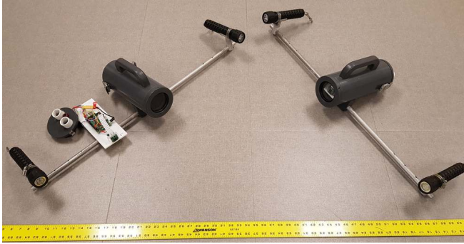
Fig. 6. Underwater cooperative localization nodes with dive lights.
