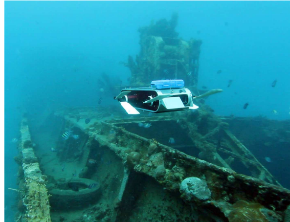
Figure 2: An Aqua underwater robot collecting data over a shipwreck.
