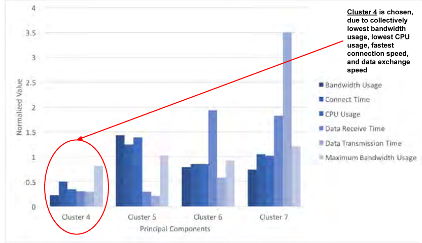
Figure 21: Chosen cluster in Group-B, by the Optimal Scheme Decider
