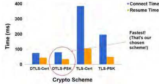
Figure 15: Time for connection vs. resumption for different encryption schemes. Our chosen scheme DTLS-PSK has very fast connection, and the fastest reconnection, due to Session Resumption support
