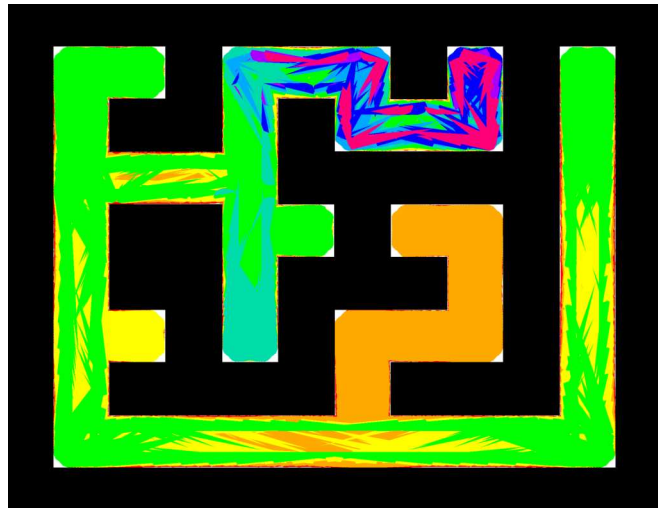
Fig. 1. A maze-like environment. Our algorithm generates plans that are guaranteed to cover particular regions of the environment. Results from several runs of the algorithm, showing the region guaranteed to be covered by the plans for error bounds ranging from 0.5 degrees to 4.5 degrees of error on each motion, are shown in corresponding colors: 0.5°, 1°, 1.5°, 2°, 2.5°, 3°, 3.5°, 4°, and 4.5°. Layers are stacked by increasing error because the lower (more precise) layers cover everything the layers above them cover. For example, very little red is visible because very little area covered at 0.5 degrees is not also covered at 1 degree.
