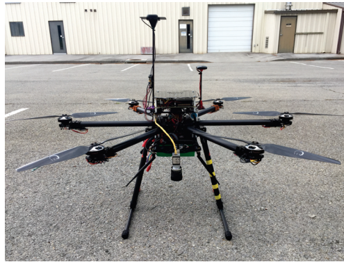
Figure 2. A custom unmanned aerial vehicle shown with the first-generation Swifnav Piksi RTK GPS unit.
