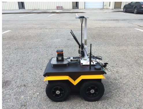
Figure 1. The Jackal unmanned ground vehicle shown with the first-generation Swifnav Pixi real-time kinematic global positioning system (RTK GPS) unit.
