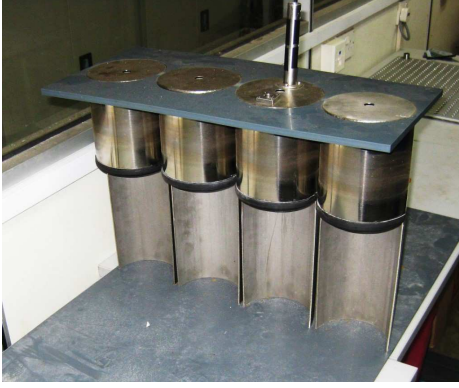
Fig. 2: Left: A row of four OWC-piles before its deployment in the wave flume. Right: a sketch of a single OWC-pile.
