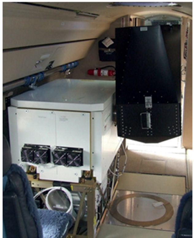
FIG. 2. Photos of (top) HCR on the wing of GV and (bottom) HSRL pointing (left) up and (right) down inside the GV.
