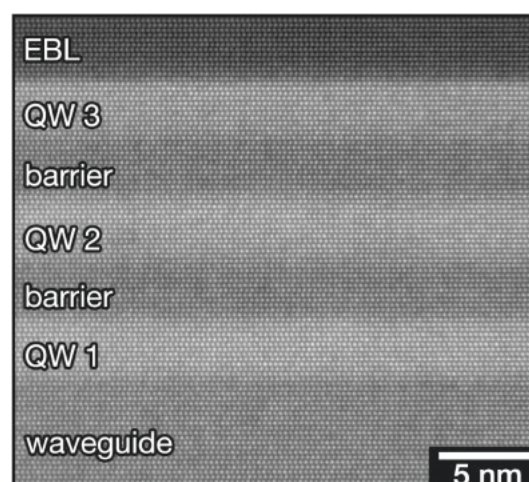
Fig. 1. STEM image of an Al 0.55 Ga 0.45 N/Al 0.65 Ga 0.35 N MQW structure with an EBL. All wells and barriers are well-defined and of homogenous composition.
