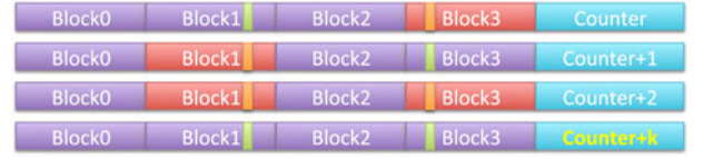
Fig. 2. Counter advance example. Green indicates a SA-R fault and orange a SA-W fault. Purple blocks are error free and red blocks contain an error.
