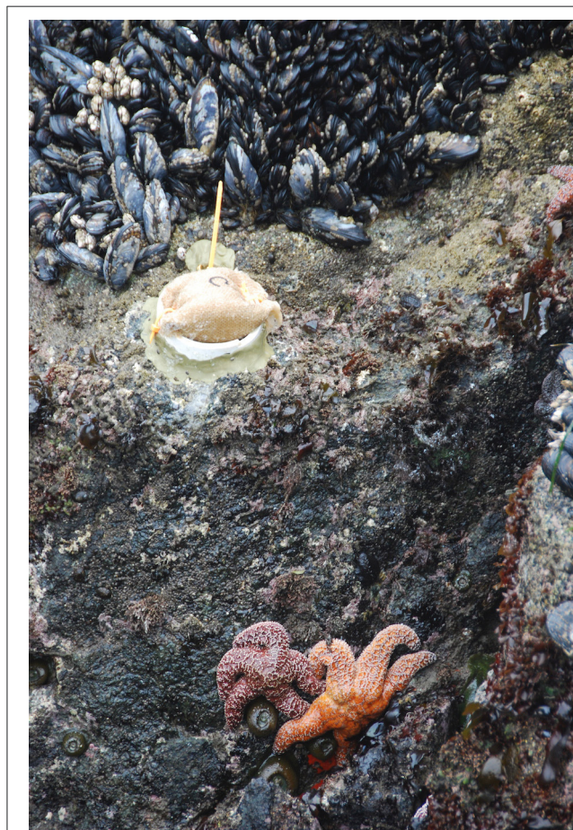
FIGURE 4 | A “robosetstar” biomimic deployed in the intertidal next to live seastars ( Pisaster ochraceus ) and their mussel prey. An iButton temperature logger is embedded within the foam and the unit is affixed to the rock using marine epoxy.
