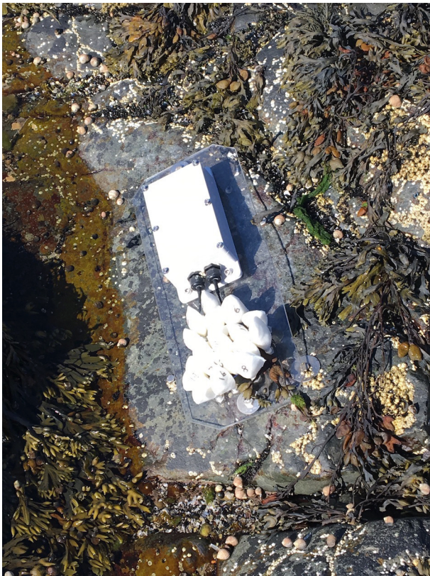
FIGURE 7 | A robomussel bed prototype deployed in the rocky intertidal zone in Nahant, MA USA. The robomussels in this prototype are colored white in order to collect preliminary data on how albedo may affect the accuracy of biomimetic devices.
