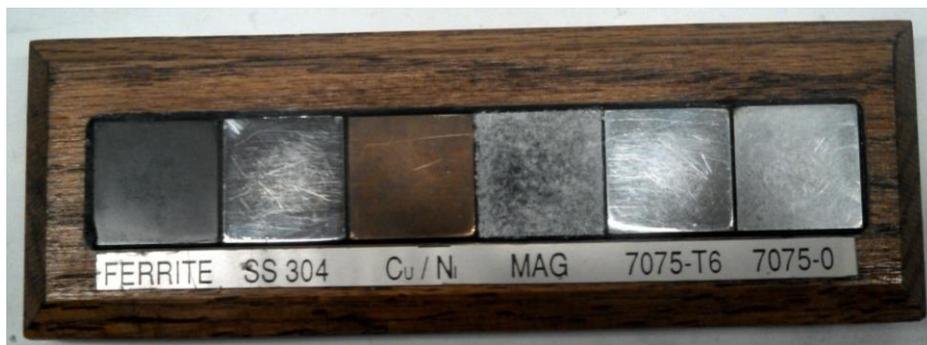
**Figure 1: Standard conductivity samples used for lift-off and conductivity assessments.**
