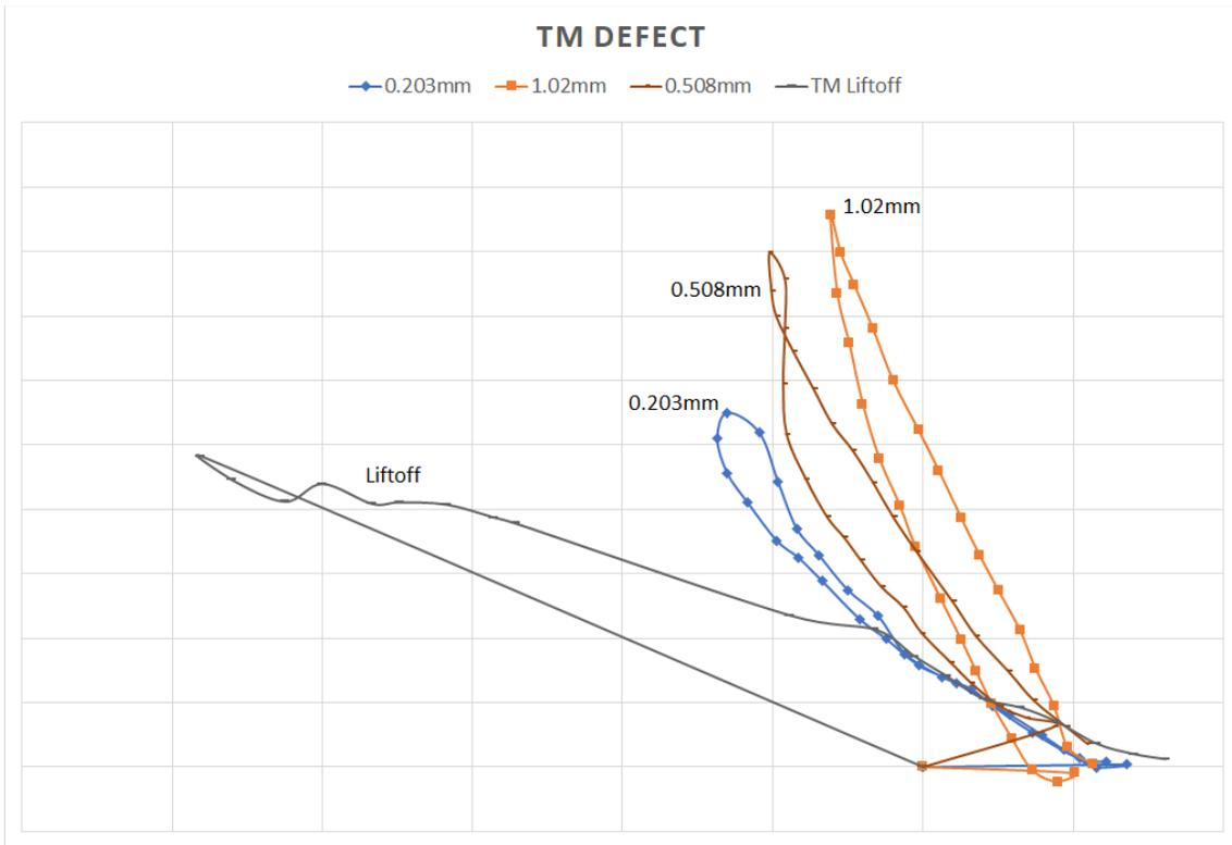
**Figure 6: Results of the surface-breaking defects (cracks) in TM SS 17 4 PH sample using 500 kHz absolute frequency probe.**
