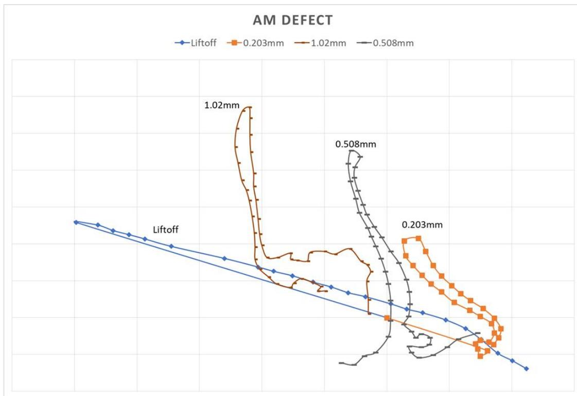
**Figure 7: Results of the surface-breaking defects (cracks) in AM SS 17 4 PH sample using 500 kHz absolute frequency probe.**
