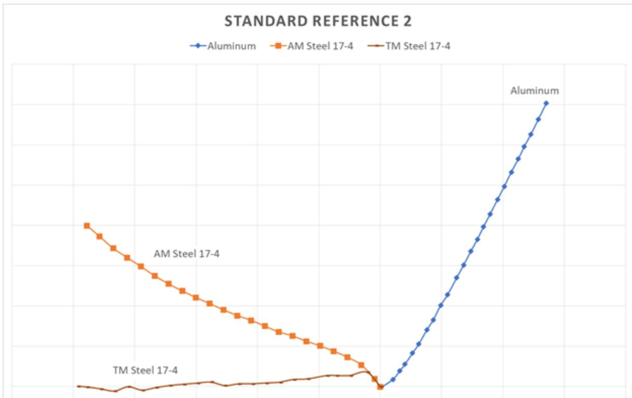
**Figure 5: Lift-off curves for comparison of the conductivity for a non-magnetic material (Aluminum) as well as TM and AM SS 17 4 PH samples.**
