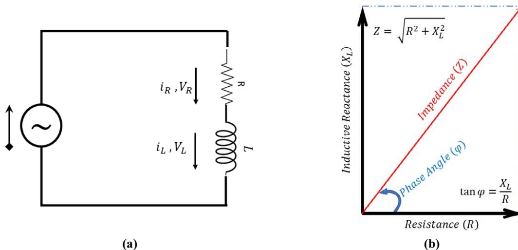
**Figure 3: Eddy current electromagnetic testing method (a) circuit diagram of an eddy current inspection system, (b) impedance plane.**
