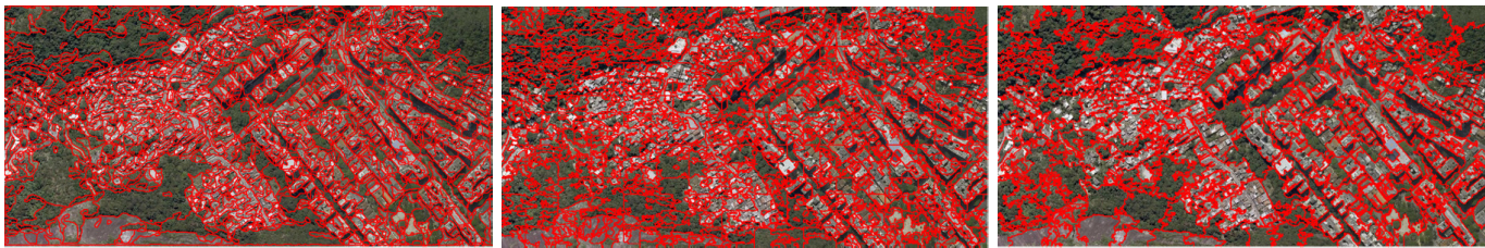
Fig. 3. Superpixel maps obtained from OWT-UCM (left), SLIC (middle) and LSC (right) segmentation methods.
