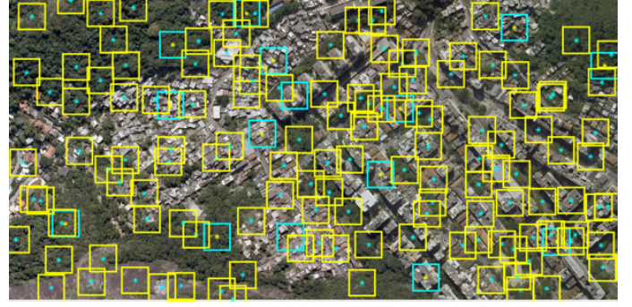
Fig. 2. Illustration of the rectangular patches created for deep superpixel feature extraction. The cyan windows around yellow crosses ( i.e. expert labeled points) represent the patches that are used to train the classifier. The yellow windows around cyan stars ( i.e. centers of the superpixels) represent the patches that are used to receive the superpixel-level label.
