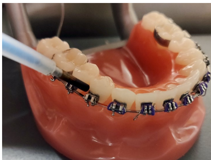
Figure 1. Near-infrared (NIR) scanning fiber endoscope (SFE) prototype on a typodont with orthodontic appliances.
