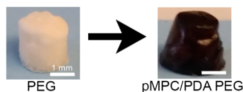
Figure 1. Photographs of a PEG hydrogel before and after pMPC/PDA functionalization. Scales bars are 1 mm.
