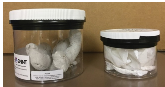
Figure 18. Photograph of 500-mg sample of as-received BNNT (left) and 500-mg sample of BNNT following purification at the National Institute of Aerospace (NIA) at 600 °C for 1 h (right).
