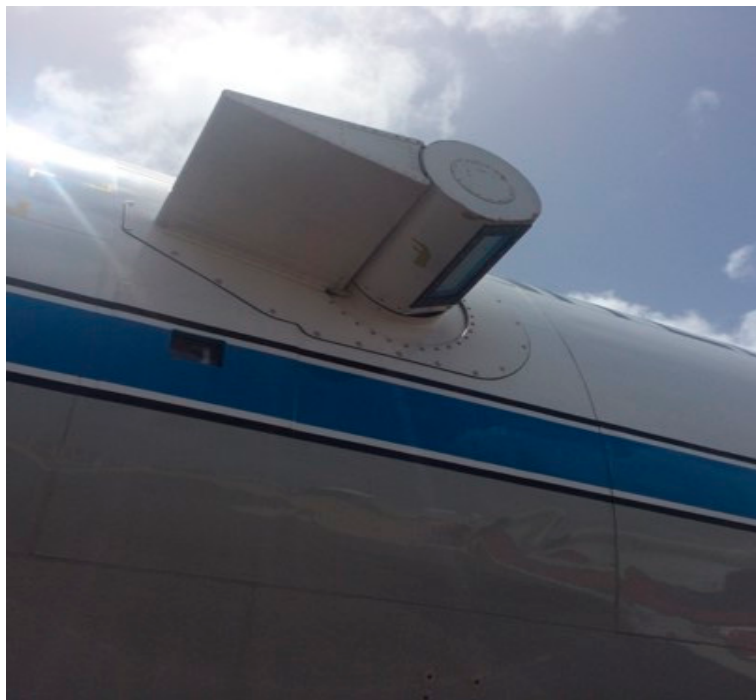
Figure 1. P3 Doppler Wind Lidar (DWL) bi-axis scanner.
