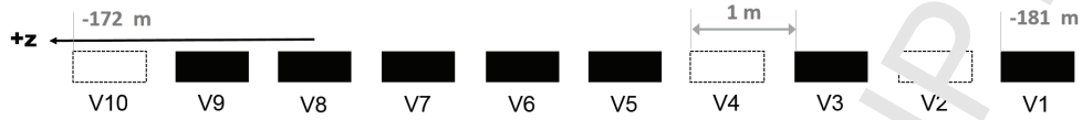
Figure 4: Diagrammatic view of the Vpol trigger array. Ten Vpol antenna units, shown in Fig. 5b, were deployed at 1 meter spacing starting at a depth of 181 m. Three of these units proved inoperative after deployment, shown as unshaded, leaving 7 non-uniformly spaced antennas for the beamforming trigger. Not shown here are the deployed Hpol antennas at -183 m and -185 m, which are not part of the beamforming trigger.
