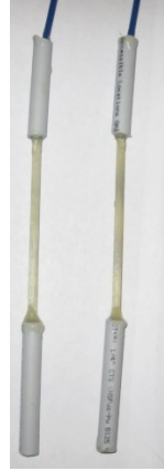
(a) Schematic view (b) GFRP-packaged FBG sensors (c) Representative specimen Fig. 10 Test specimen and instrumentation
