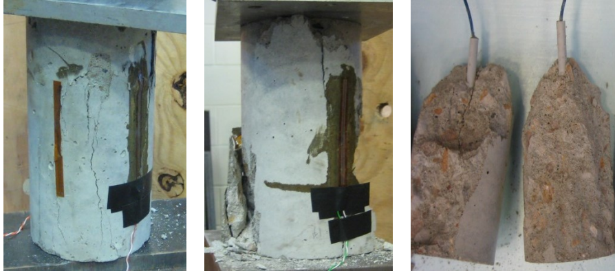
(a) Crack initiation (b) Failure mode (c) Tested specimens Fig. 14 Concrete behavior of the tested specimens
