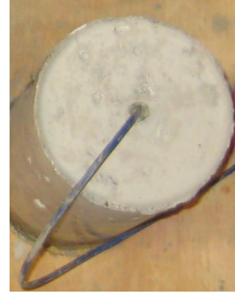
(a) Schematic view (b) GFRP-packaged FBG sensors (c) Representative specimen Fig. 10 Test specimen and instrumentation
