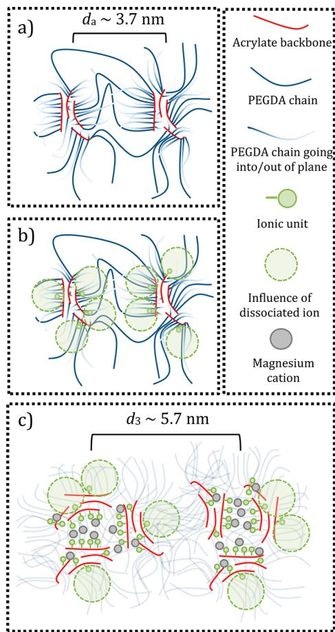
**Figure 4.** Schematic detailing proposed morphology of (a) pure PEGDA/PEGDMA films, (b) unaggregated films containing ionic units, and (c) aggregated ionomer films. Pictured as a two-dimensional representation, chains with a color gradient are going into and out of the plane. For clarity, PEG chains are lightened in box c.
