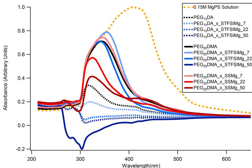
Figure 8. UV/vis absorption spectra of polysulfide crossover solutions for  $\text{PEG}_{20}\text{DMA}$  and  $\text{PEG}_{13}\text{DA}$  films of varying Ch:EO and anion chemistry.
