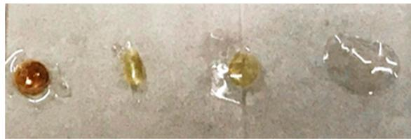
Figure 9.  $\text{PEG}_{13}\text{DA}$  films recovered from diffusion cell experiments. From left to right Ch:EO is 0, 7, 22, and 50.
