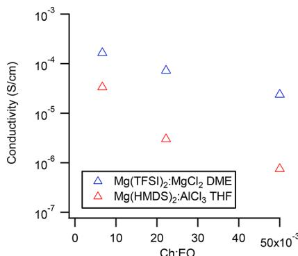
**Figure 6.** Conductivity of  $\text{PEG}_{13}\text{DA}_x\text{STFSIMg}$  films swelled with two electrolytes relevant for Mg–S batteries.
