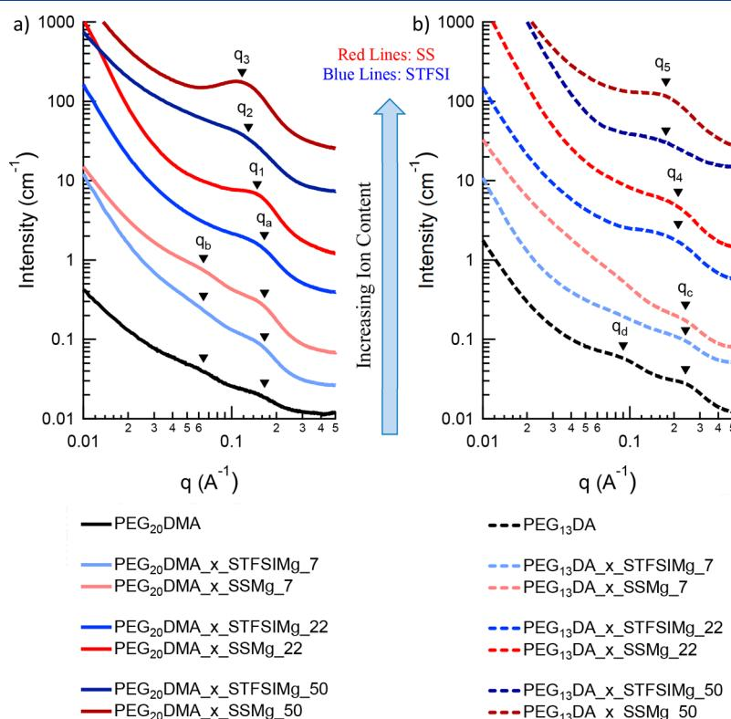
Figure 3. SAXS spectra for  $\text{PEG}_{20}\text{DMA}$  (a) and  $\text{PEG}_{13}\text{DA}$  (b) ionomers of varying anion chemistry and Ch:EO. Samples are swelled in THF and analyzed at room temperature (23 °C). Spectra are shifted vertically for clarity.
