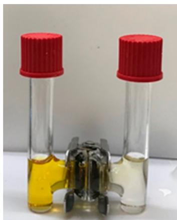
**Figure 7.** H-style diffusion cell containing MgPS in a THF-based electrolyte on the left-hand side, the same electrolyte without added sulfur on the right-hand side, and the film to be tested in between. Pictured is the H-cell containing a  $\text{PEG}_{20}\text{DMA}$  film 2 h after assembly.
