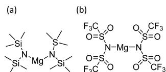
Figure 2. Magnesium electrolyte salts (a)  $\text{Mg}(\text{HMDS})_2$  and (b)  $\text{Mg}(\text{TFSI})_2$ .
