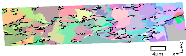
Figure 4. Grain map representing microstructure of PS-PI/d-PS (10 wt %) annealed at 130 °C for 3 days. Random (gradient) color assignment is used to distinguish adjacent grains with misorientation exceeding 15^\circ ; the x - and y -axes represent the in-plane and out-of-plane (i.e., normal to substrate) orientation of the film. HAGBs with misorientation angle \theta > 60^\circ are highlighted with thick black lines.
