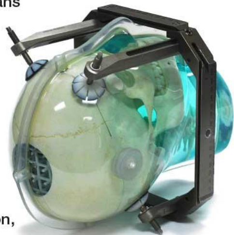
Inter-cranial Grid Phantom 335 Physical Control Points
