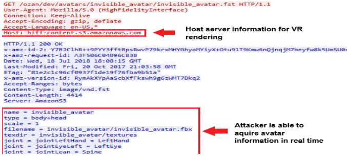
Fig. 9: Packet Sniffing using Wireshark showing avatar and host server information getting disclosed.
