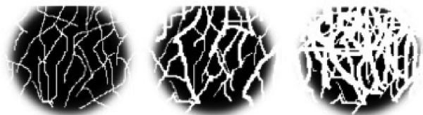
Figure 3: Growing of micropores and mesopores under steam activation process.
