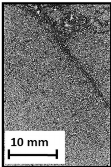
Fig. 11. Scanned thin section of the sample that deformed under an effective pressure of 150 MPa.
