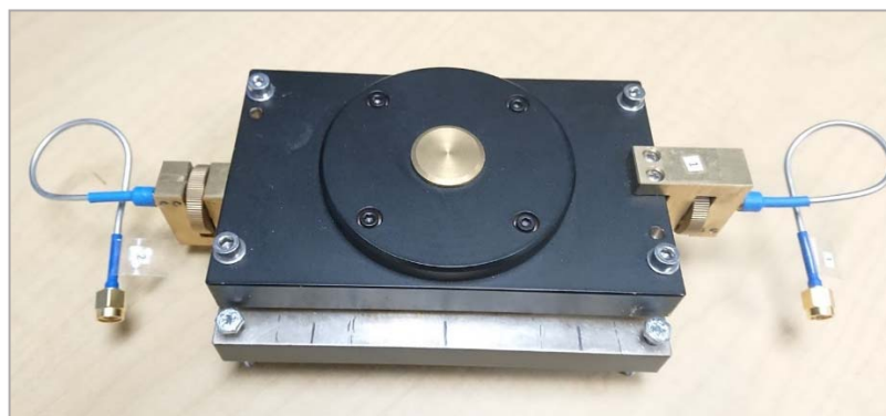
Figure 2. Image of a split post dielectric resonator.
