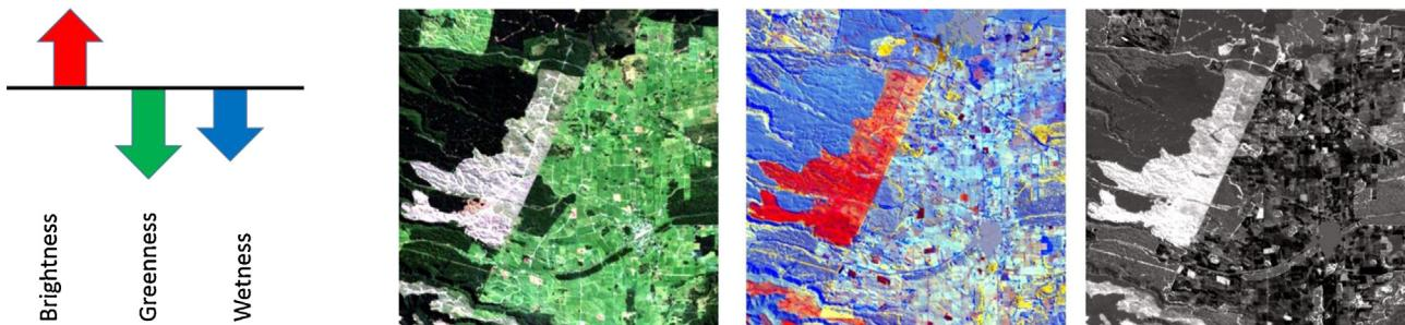
**Fig. 4.** From left to right, there are the conceptual diagram of the forest disturbance index, a true color example of a forest disturbance, a tasseled cap image of the same disturbance and the resulting disturbance index image.
