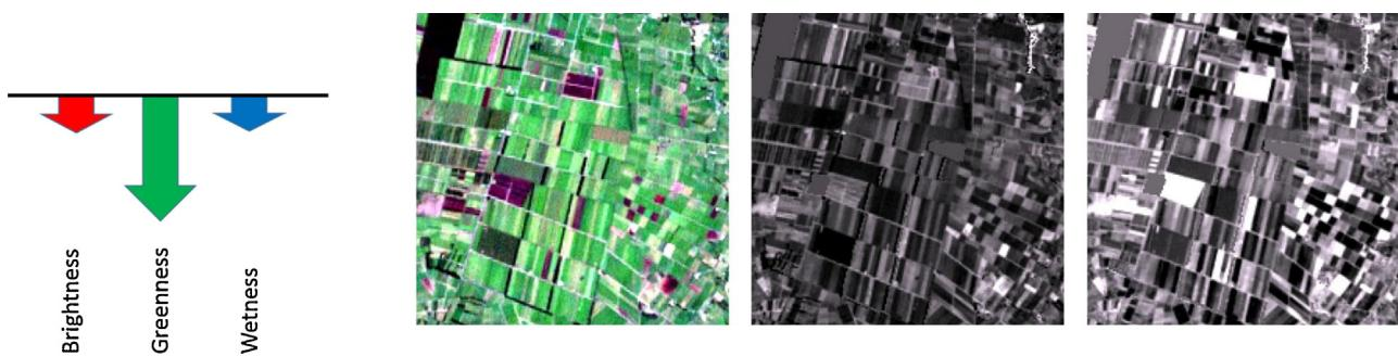
**Fig. 5.** From left to right, there are the conceptual diagram of disturbed (grazed) grasslands, a true color example of a partially grazed grassland, an example of the disturbance outcome when the original disturbance index is used and an example of the adjusted disturbance data.
