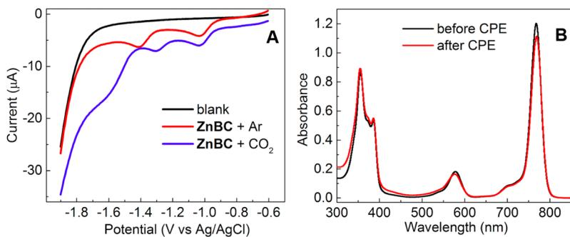
**Figure 2.** (A) CV scans of electrolyte solution without catalyst ZnBC (black), with ZnBC under an argon atmosphere (red), and with ZnBC under a CO<sub>2</sub> atmosphere (blue). Only cathodic traces are displayed for clarity. (B) Absorption spectra of the electrolyte solution before (black) and after (red) 4 h of CPE. The same amounts of aliquots from the electrolyte solution were used.
