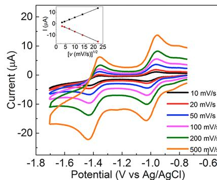
**Figure 1.** Scan-rate-dependent CV of 0.5 mM ZnBC in DMF with 5 M H<sub>2</sub>O. Inset: square root of scan rate versus current for the first reduction peak.
