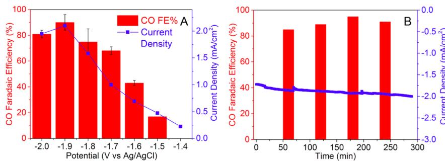
**Figure 3.** (A) CO Faradaic efficiencies and total current densities at various potentials (averaged from two measurements). (B) CO Faradaic efficiencies and total current densities after 1, 2, 3, and 4 h of electrolysis at  $-1.9$  V vs Ag/AgCl. H<sub>2</sub> gas is the only other reduction product in all measurements.
