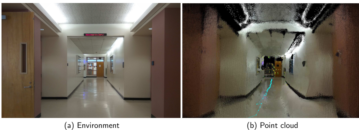
Figure 16. 3D mapping (point cloud) results of the indoor corridor.
