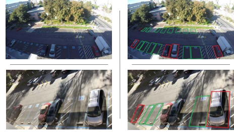
Figure 7. Input Image To The Model and The Output Image Indicating the Vacant and Occupied Parking Slots at SJSU 20Min Parking lot .
