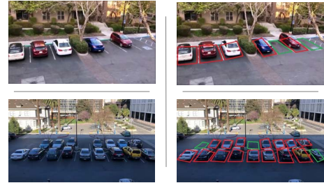
Figure 8. Slot Occupancy detection results at Avalon on the Alameda(above) and SJSU south garage(below) Parking lots
