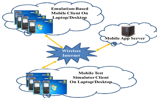
(a) Large-scale Emulation-Based or Simulation-Based Mobile Test Infrastructure
