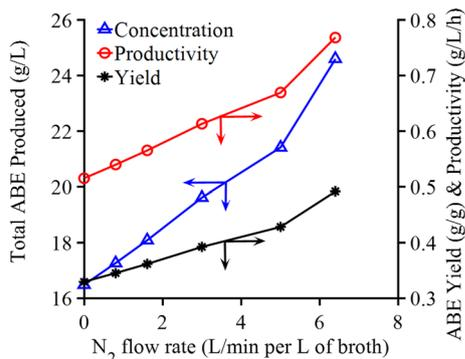
**Fig. 6** Total ABE produced (total concentration in the fermenter and stripped stream), productivity and yield from the simulated batch ABE fermentation and in situ gas stripping with different gas flow rates
