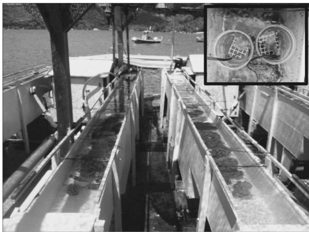
**FIGURE 2 |** Picture of flumes with experimental coral reef communities 1 and 2 in place. Covers with blue filters are not in place so as to show coral reef community within the flume. Inset shows 2-L chamber, containing a *Pocillopora verrucosa* colony and a small pump for seawater circulation, which were placed within the flumes at the time of incubation.
