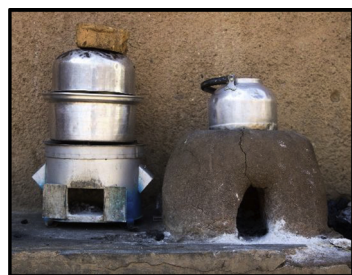
Fig. 2. CHARCOAL BURNING HOUSEHOLD COOKSTOVES EVALUATED IN LIRA, UGANDA. From left to right: ILF Improved Charcoal Stove, Traditional Mud Charcoal Stove. (Photo credit: Nick Moses).
