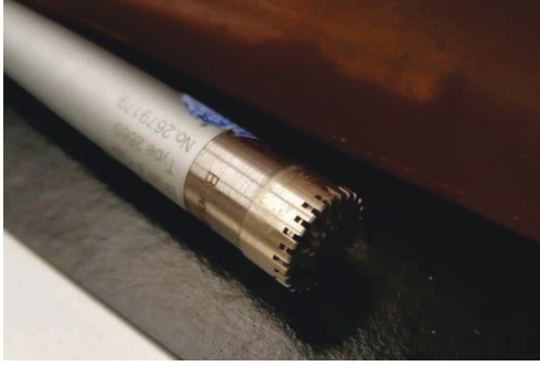
Fig. 9: A B&K Type 4940 1/2 inch microphone used in the streamwise array to measure the wall jet background noise. Shown equipped with a factory-made salt-and-pepper cap to protect the diaphragm.
