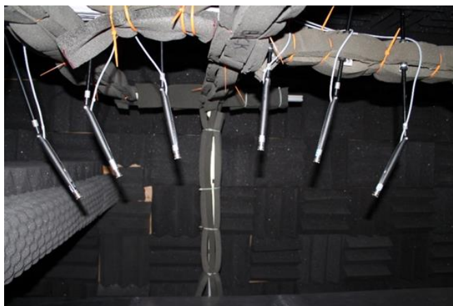
Fig. 8: Streamwise array of B&K ½ inch microphones arranged in an arc-like sketch to capture background noise contamination around the wall jet testing area. The 609mm radius setup is shown.
