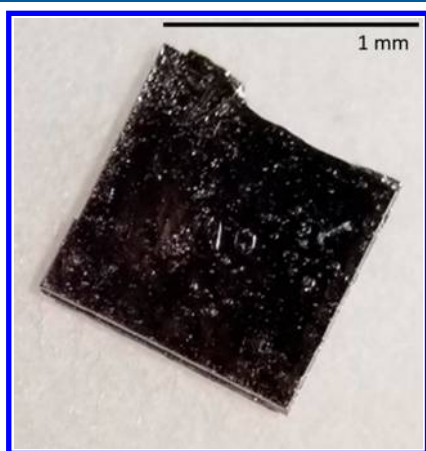
Figure 1. Photograph of a typical crystal of \text{Ce}_6\text{Co}_5\text{Ge}_{16} . Crystals are typically well-faceted square plates ranging in size from \sim 0.2 to \sim 10 mm on edge.
