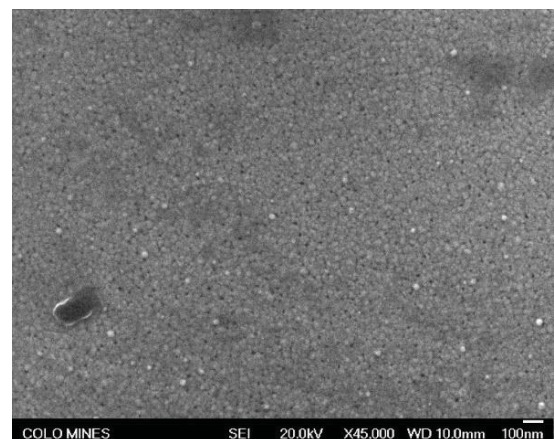
Fig. 7. SEM image of 3% ZnTe/Sb/ZnTe sample annealed at 320°C for 1 hr.
