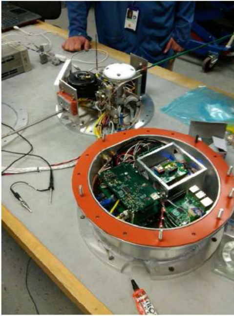
Fig. 1. NASA USIP sounding rocket payload. The TDIP is the visible top board in the electronics stack, shown in the bottom canister. The probe arms are shown extending out of the top canister in the picture.
