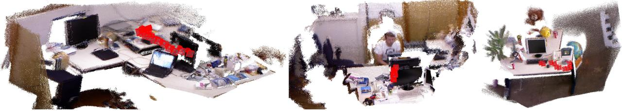
Figure 5: Results for the 3D point-cloud registration, using the TUM RGB-D data-set [39]. We use three different sequences of 3D scans, freiburg1\_room (at the left), freiburg1\_xyz (at the center), and freiburg2\_desk (at the right) and the method described in the paper to compute the relative transformations between the cameras. In these figures we show the registration of 100 RGB-D scans.
