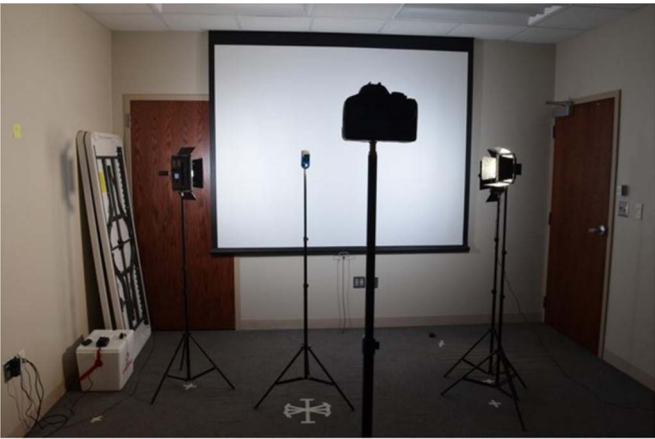
Fig. 3. Photography setup showing lumen meter collecting data.
