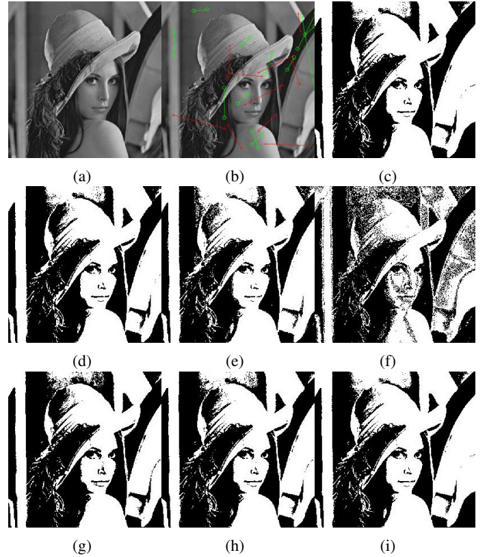
Fig. 6: Image segmentation: (a) original image; (b) original image with feature constraints; (c) accurate segmentation; approximate segmentation for (d) p=2 ; (e) p=8 ; (f) p=14 ; and approximate segmentation using the proposed method for (g) p=2 ; (h) p=8 ; (i) p=14 .
