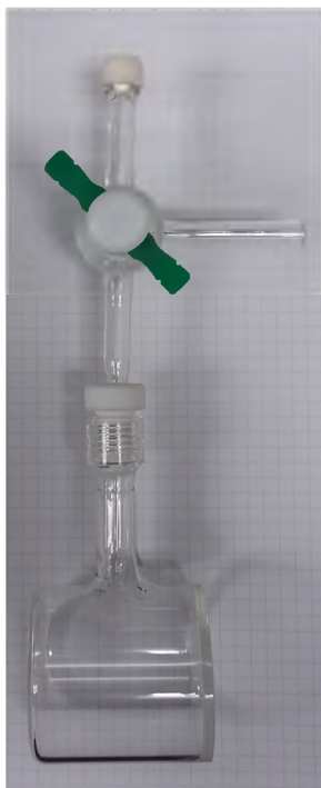
Figure 1: Photograph of the 2" diameter x 2" length borosilicate glass test cell with purge and septa ports.
