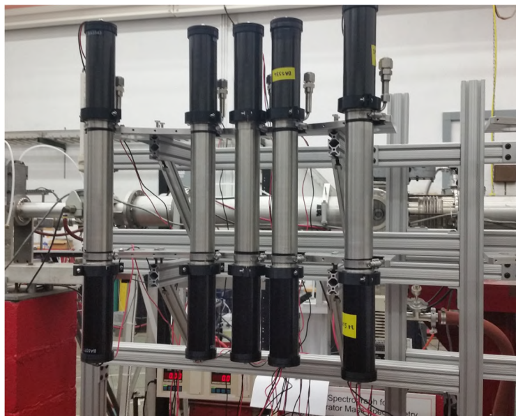
Figure 10: Photograph of the SABRE detectors set up in a neutron spectroscopy configuration at the Nuclear Science Laboratory at the University of Notre Dame, for a neutron spectroscopic measurement. The Swagelok expansion port is just visible at the top of each bar, demonstrating how the design protects against light loss due to any expansion bubble.
