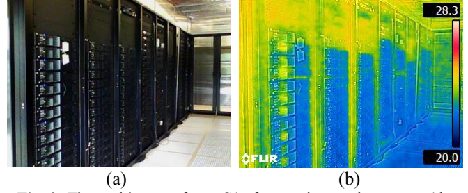
Fig. 9: Thermal image of row C1 after turning on the servers (the second steady state) in scenario 3.
