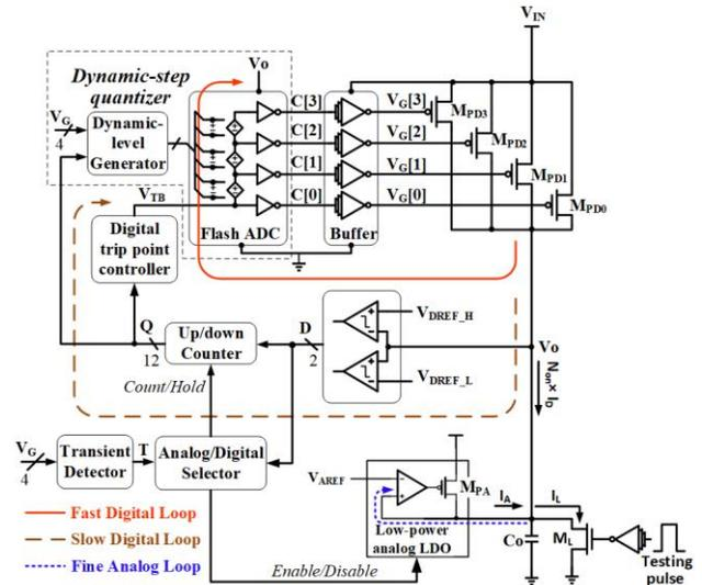
Fig. 1. System architecture of the proposed LDO
