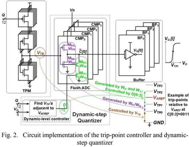
Fig. 2. Circuit implementation of the trip-point controller and dynamic-step quantizer
