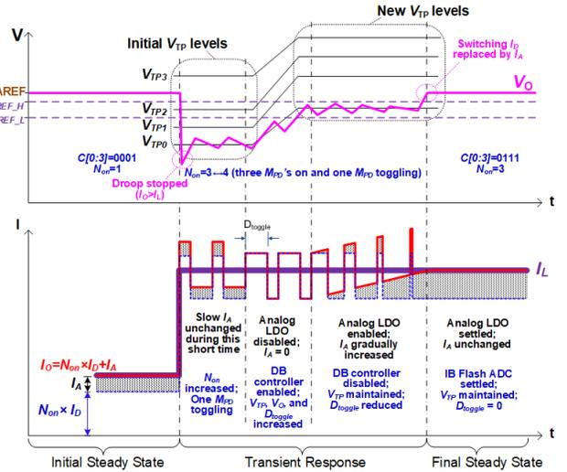
Fig. 4. A transient example for  $C[0:3]$  changing from 0001 to 0111
