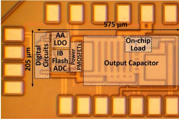
Fig. 5. Micrograph of the fabricated chip
