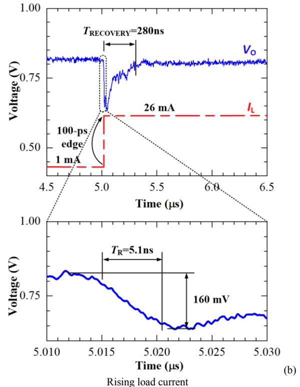
Fig. 7. Measured transient response
