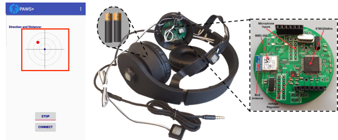
Fig. 1. Left: UI of PAWS. When a car is detected, a dot corresponding to the relative position (direction and distance) of the car is shown in the graph highlighted in red. Right: low-power embedded headset, introduced in [1], that is used for car direction estimation.
