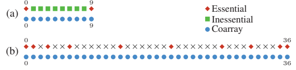
Fig. 1. The array geometries and the nonnegative parts of the difference coarrays for (a) ULA and (b) MRA. These arrays have 10 physical sensors.
