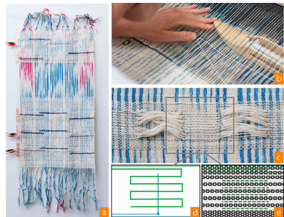
Figure 1: AdaCAD supports the design of woven smart textiles by augmenting traditional weaving drafts with smart textiles specific operations and views. We used the tool to create a prototype we developed with multiple regions of touch sensing and color change (a, b, c). AdaCAD allowed us to view the design as yarn paths (d) or traditional weaving drafts (e).
